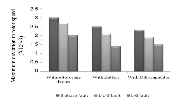
Comparison of impacts of storage devices on rotor speed deviation
